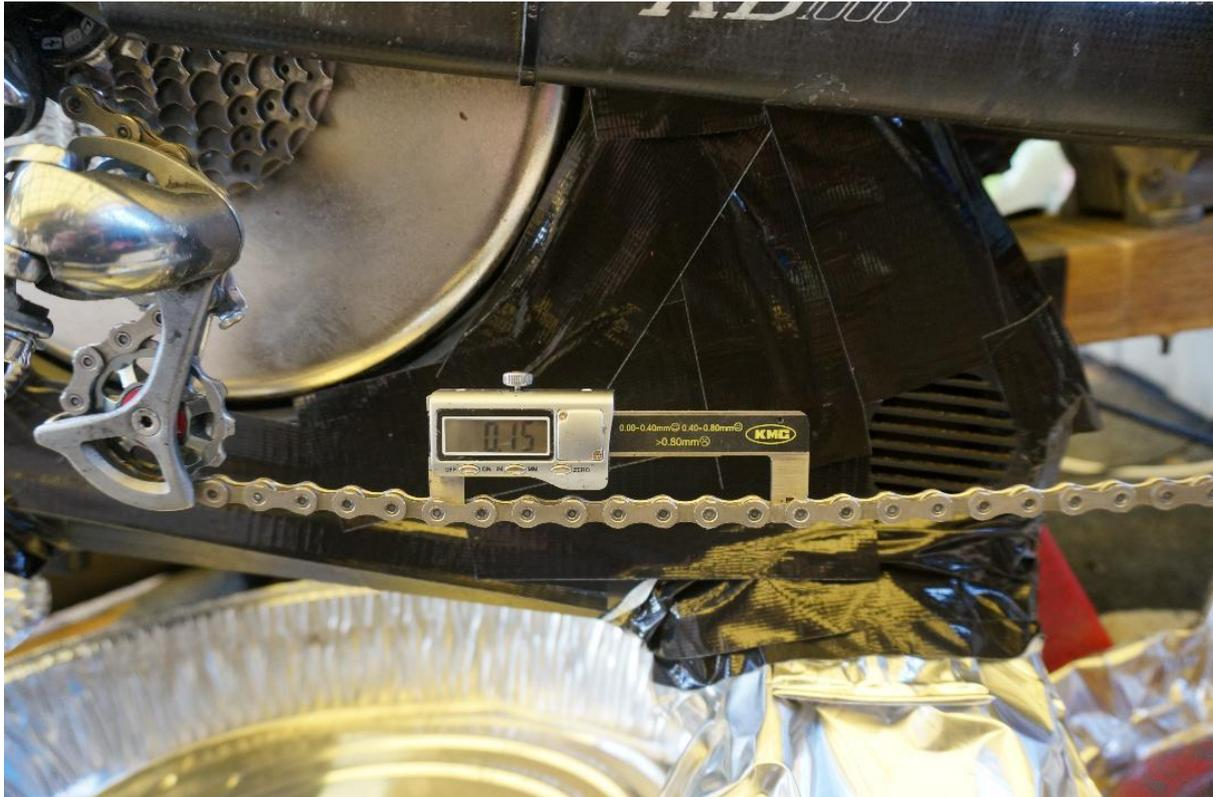
(Chain wear checker used by ZFC – by far the best in the world – can check and re check sections of chain to same 0.01mm accuracy every single time)
