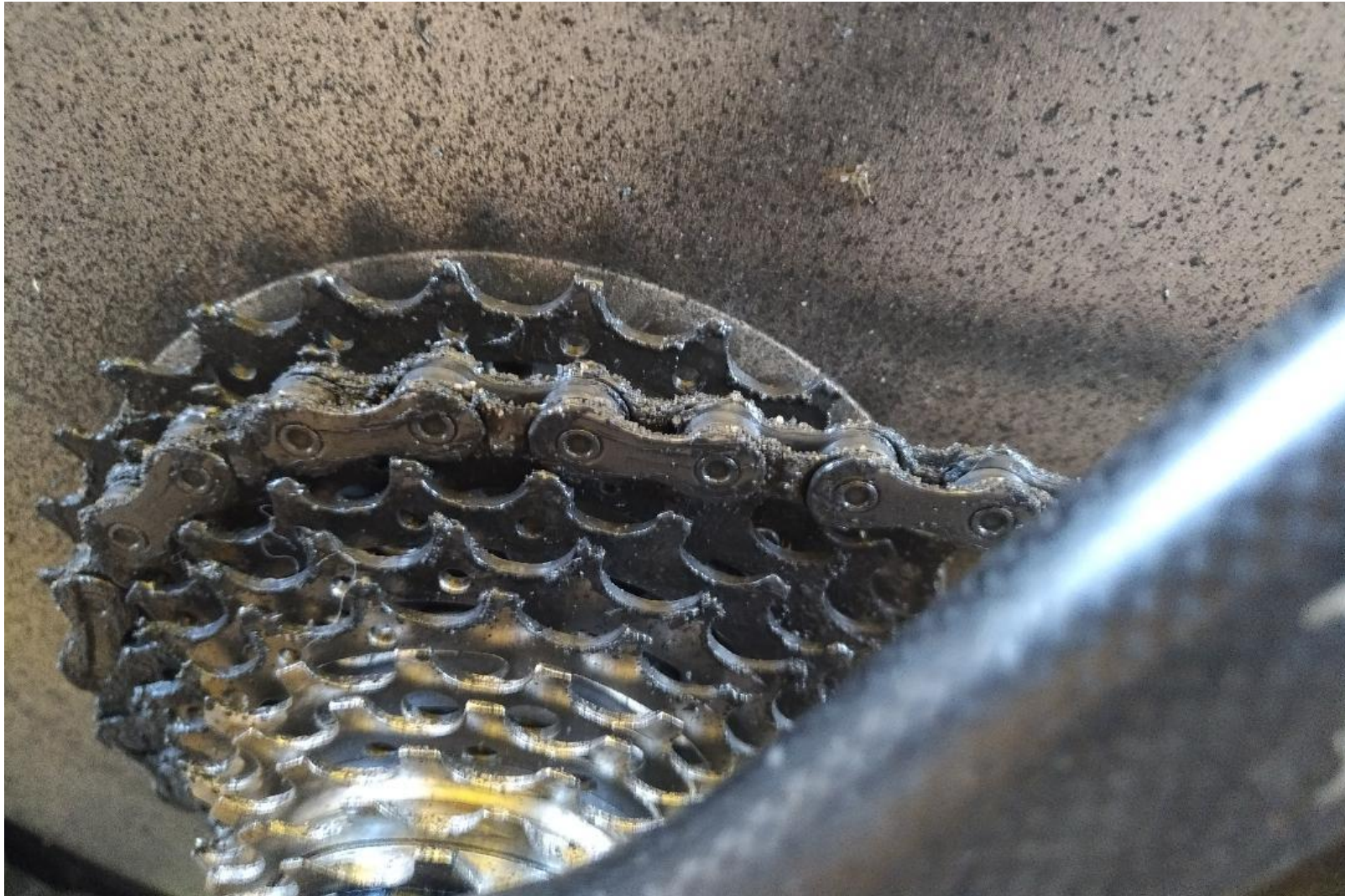
End of main test – 2000km – You can see the grit stuck in the gunk build up.
