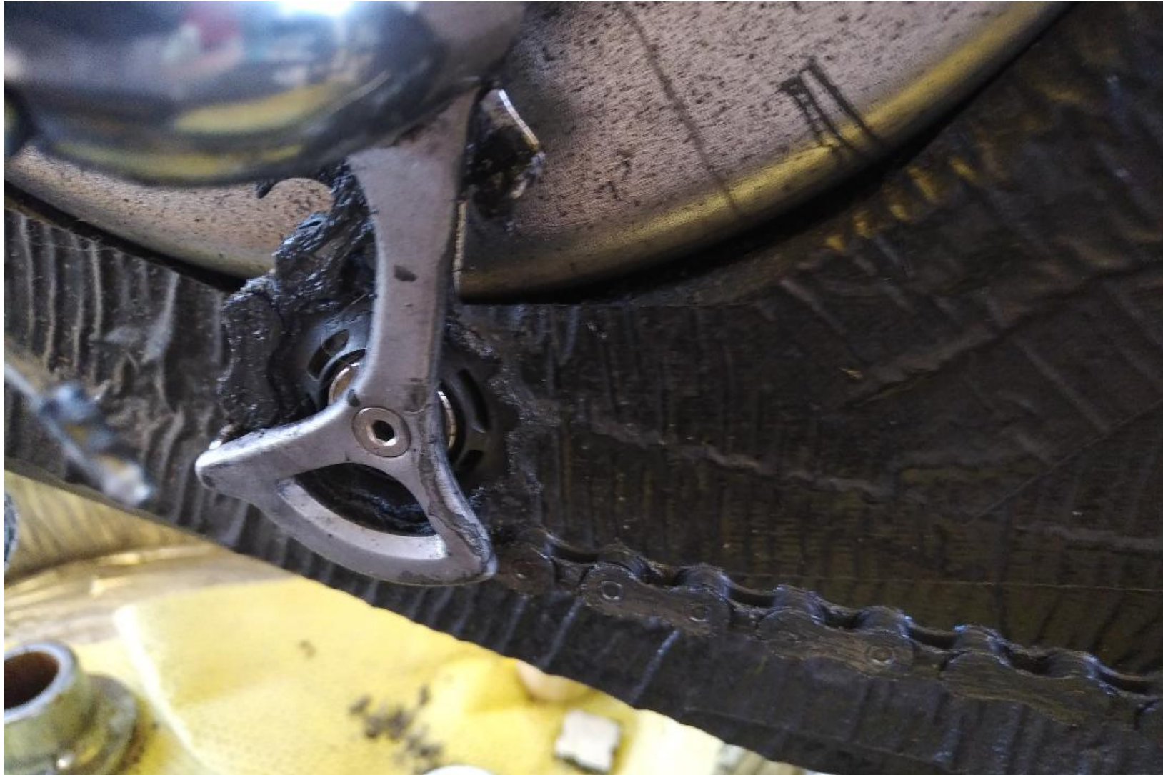
End of test – 2000km mark – It's just messy, messy stuff – the test ending at 2000km is much sooner than most other lubricants and yet the mess level is well ahead of most that went much deeper. You can see the spray on the flywheel. It was also sprayed on crank arm, pedal, and equipment I had in vicinity.
