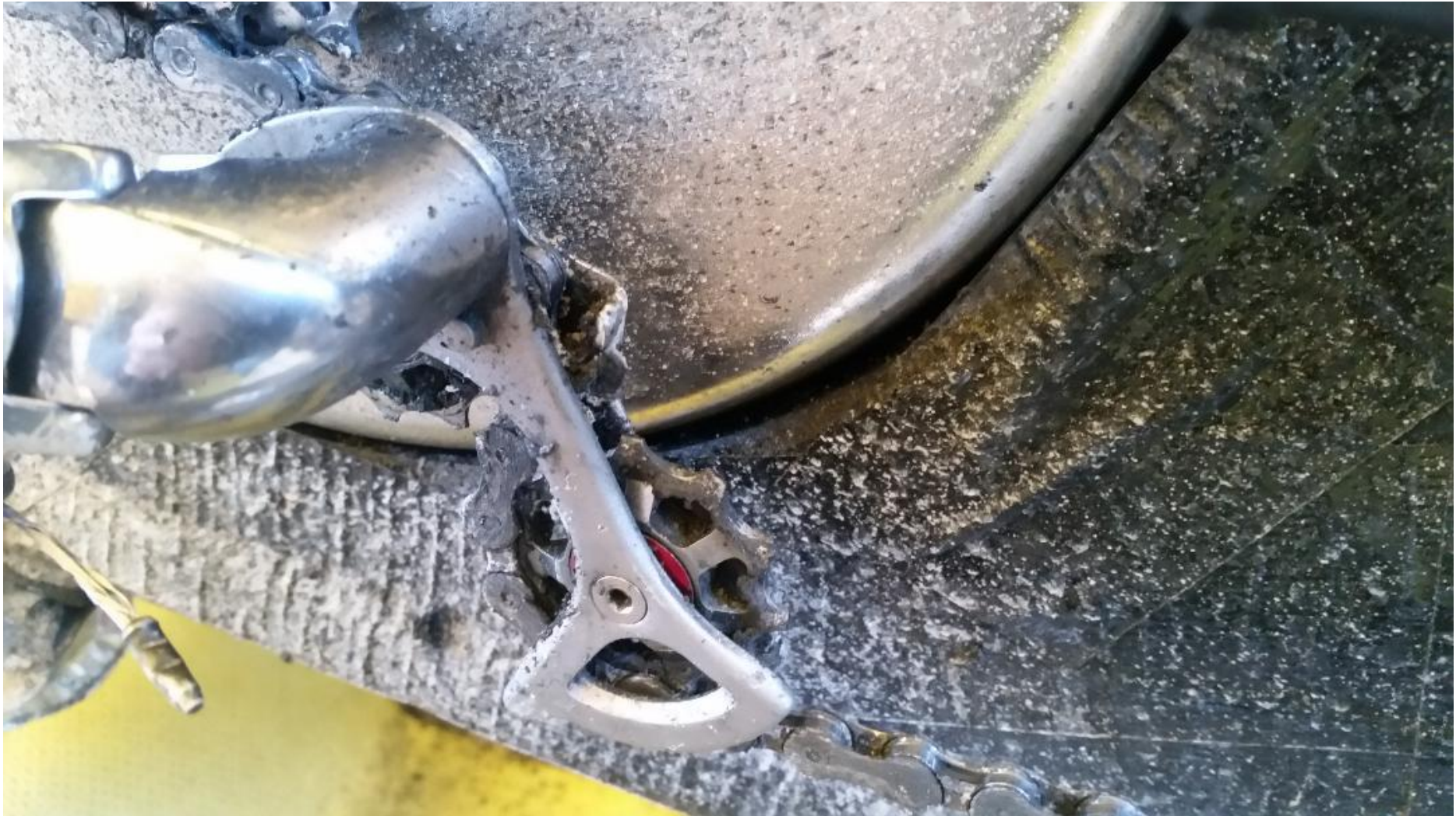
End of test – Jockey wheels – 4000km mark – in line with rest – build up here is not atrocious but it is hard to remove.
