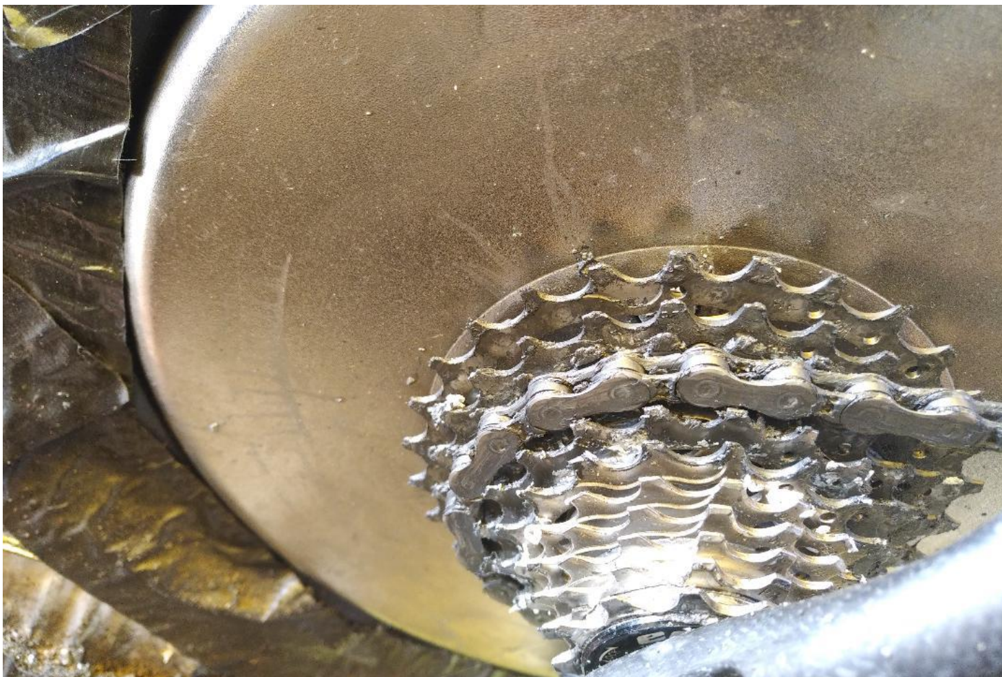
End of main test - 3000km. Pretty gunky in cassette and again, that was not easy to clean.
