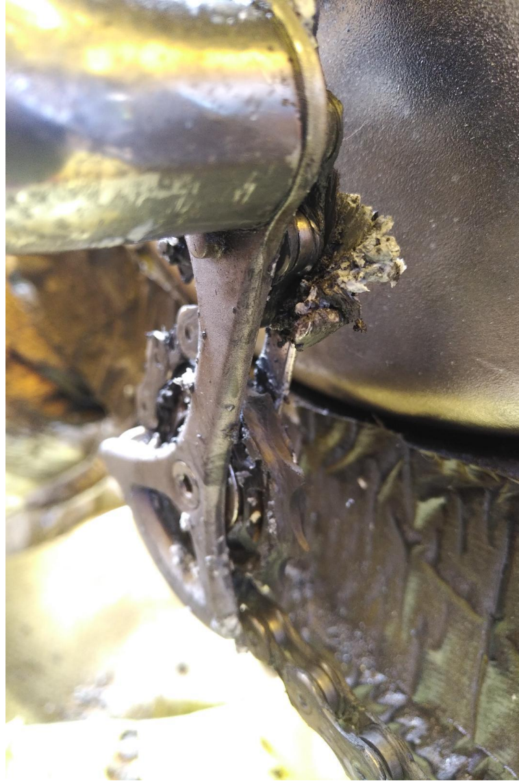
End of main test – 3000km – strangely not so bad on the actual jockey wheels, but a notable amount on cage.
