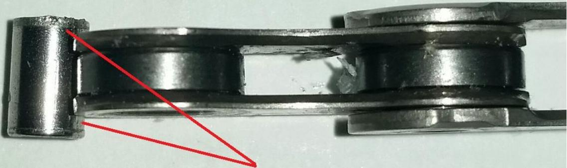
Note amount of pin width that requires lubrication - inner plate shoulders articulate around this area under full rider load.
