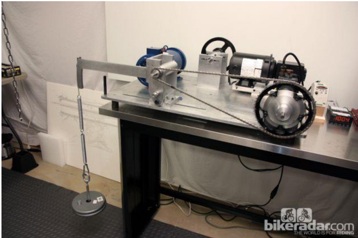
(Above – Full Tension Test Machine)
