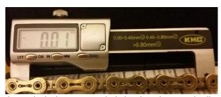
(A customers YBN ti nitride chain which chromium carbide hardened pins and rollers—checked at 3444km old — recommended replacement mark is 0.5, this is 0.01 — so 2% of wear allowance)
