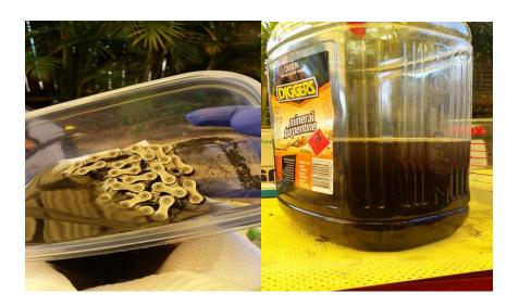
Wipe chain dry, blow chain dry hairdryer for 5 mins, now ready to wax. (note – turn wax on after chain cleaned to allow for more drying time as wax melts).
