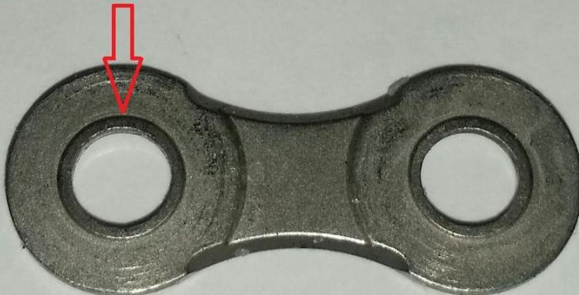
Note lubrication gap through which lubricant must penetrate & disseminate across pin width. Any contamination gathered by lubricant also needs to get back out of this gap, and back out past roller to outside of the chain.... Tricky
