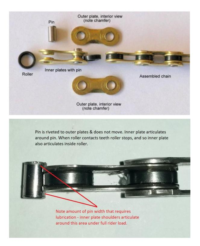
Note lubrication gap through which lubricant must penetrate & disseminate across pin width. Any contamination gathered by lubricant also needs to get back out of this gap, and back out past roller to outside of the chain.... Tricky
