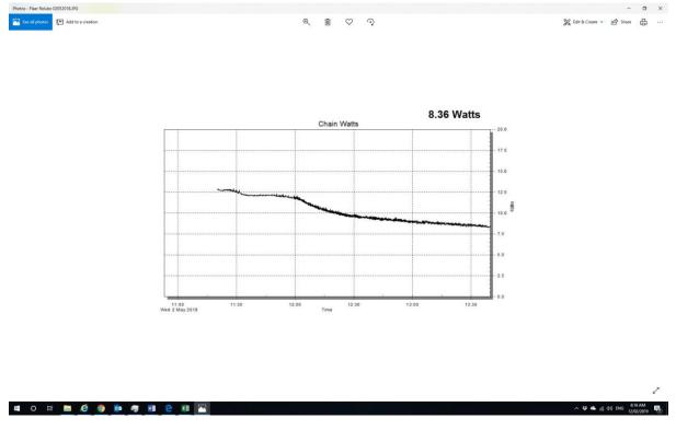
\*You can see how losses keep dropping as wax breaks in post re wax – re waxing being the equivalent of a re-lube for MSW. WLER was also re lubed. Also note that for objectivity test facility was not provided with any details re chains / lubes.
