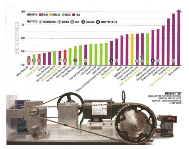
\*\*Note White Lighting Epic Ride second highest losses at just under 8w, on a perfectly cleaned chain, in a clean lab.
