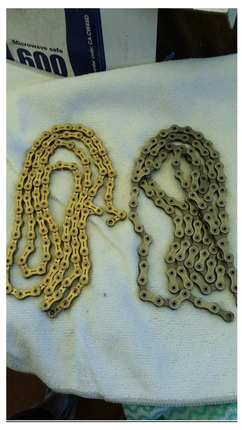
\*How clean MSW chains are after harsh conditions rides with nothing more than a quick swish in boiling water (cx race chain and oem shimano mtb training chain that came with groupset).
