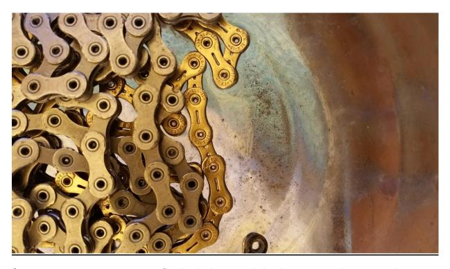
\*Note gritty contamination flushed clean with boiling water that is not being imported into wax pot.
