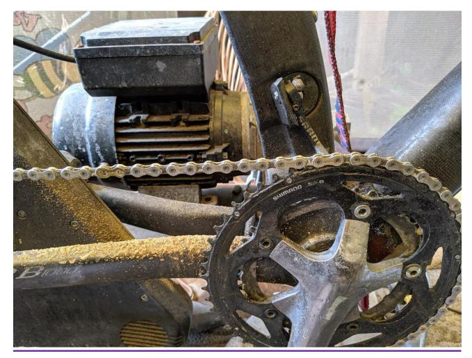
End of main test – 6000km – post extreme contamination block. Note the amount of contamination on chain stay, yet not so much on chain and chain ring.
