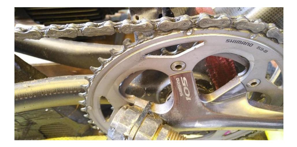
UFO Drip after 2000km. Only 11.7% of wear allowance used at this point in test. At same mark Wend had used 69.4% of allowable wear, Muc-Off Nano 145.4%. This proves UFD is not only clean on the outside, but clean on the inside where it counts. A clean chain is a fast chain. A chain whose steel components are being abraded through at a prodigious rate is obviously a very high friction & slow chain.
