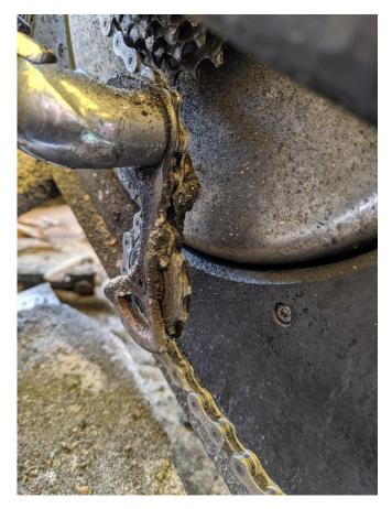
More build up of UFO D on jockey wheels vs other area's. The larger amount of ufo Drip that is applied when drizzling on led to a bit more excess build up here – in real life application you would simply wipe excess off with cloth after application, but for main test no cleaning of components is allowed to ensure like for like comparisons of lubricants with zero mainentance.
