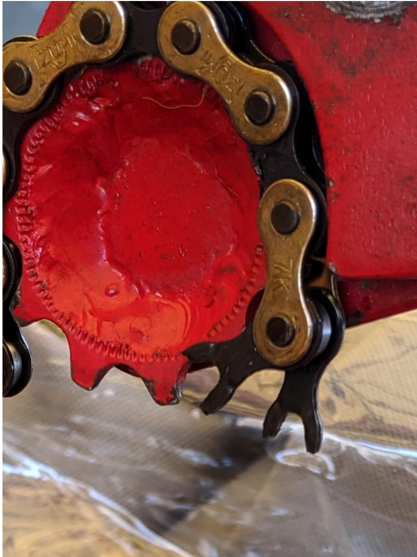
Izumi Super toughness 1/8 th track chain – after significant stretching inner plate links tore open over pin. This was repeated each test and same failure modality for Izumi Standard.
