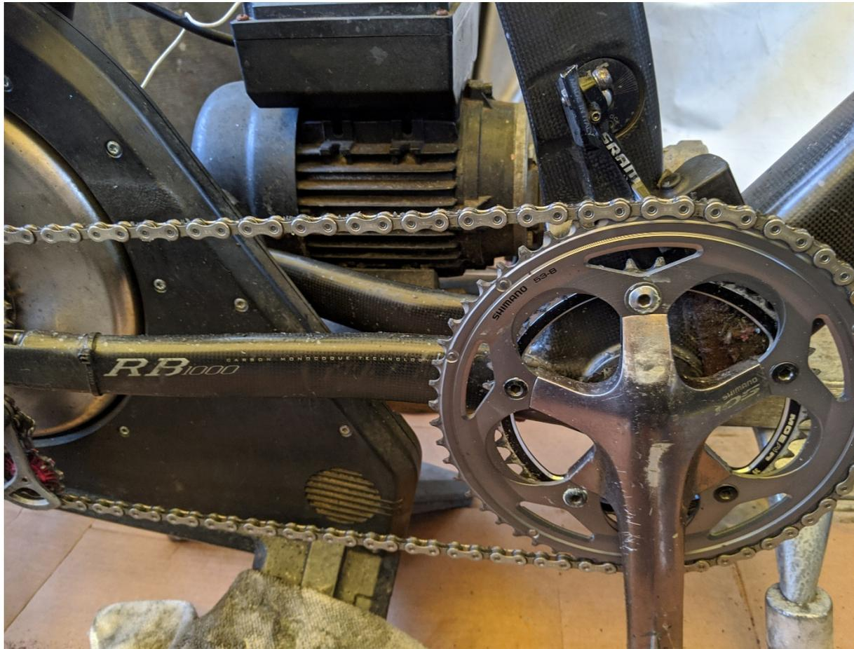
After first thousand kms and 3 applications – you can see Silca SS is exceptionally clean, this did not really change much for the next two thousand km's making it one of the cleanest drip lubes ever tested like Tru-tension Tungsten all weather and Race lubes.
