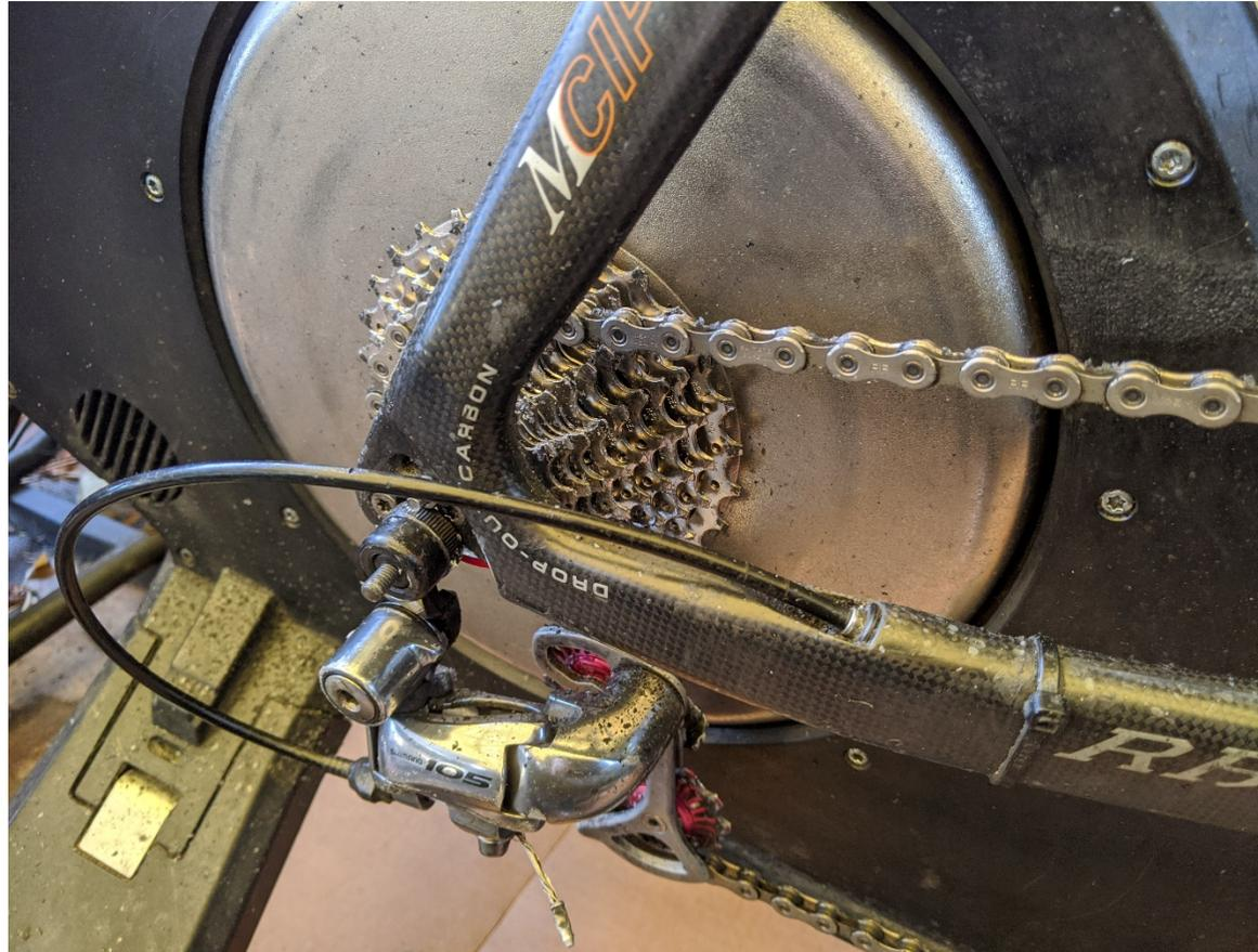
After first thousand kms and 3 applications – you can see Silca SS is exceptionally clean, this did not really change much for the next two thousand km's making it one of the cleanest drip lubes ever tested like Tru-tension Tungsten all weather and Race lubes.
