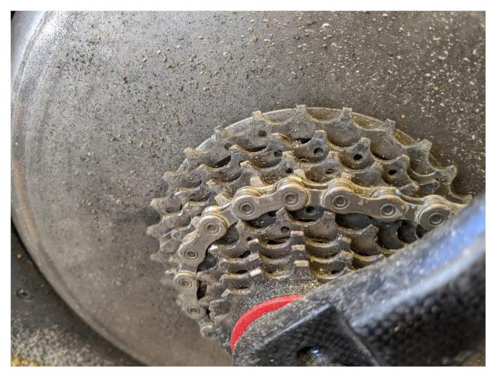
Again an impressively low build up considering 30 re lube applications and a lot of contamination thrown at chain and zero cleaning maintenance.
