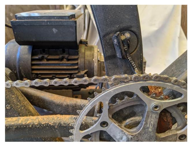
Some build up, but considering there are 30 re-lube applications if a lubricant makes it all the way to end of main 6000km test protocol.
