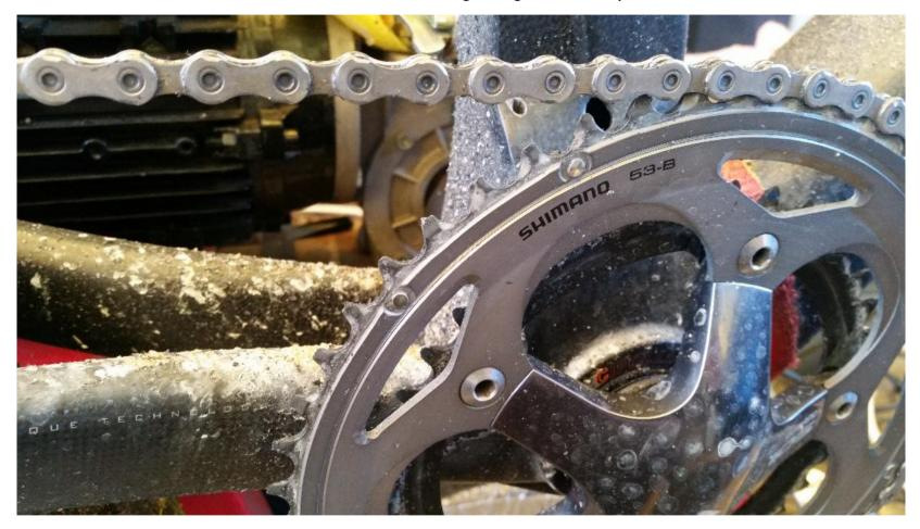
Still the benchmark due to immersive re-waxing in lab grade wax – Mspeedwax after 6000km
