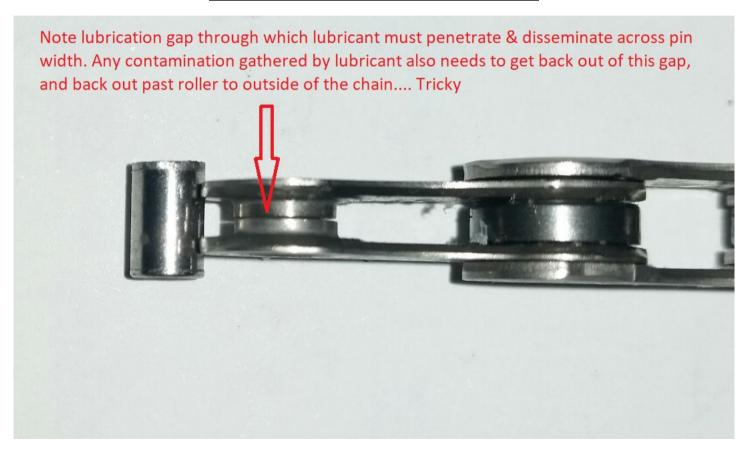
Note chamfer on outer plate. This prevents lubrication from also being able to access pin via gap between inner & outer plates, leaving the small gap underneath roller as the only lubrication gap access to pin.
