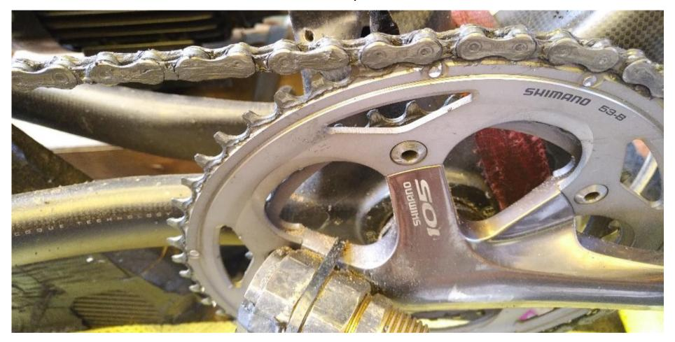
Muc Off Hydro / Nano after 2000km – 145% wear allowance at this point, Silca SS at same point – 7.5% wear.
