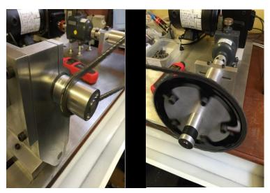
Official Outright efficiency loss if tested by dependable FTT lab: At this time I believe the official result for Hot Melt is 3.8w loss at 250w load which would make it currently the 2<sup>nd</sup> fastest lubricant known (based on outright efficiency results I can trust). UFO drip is in numero uno spot at 2.8 to 3w, Mspeedwax – original formula was 4.6w however they do have an updated formula which has also moved from Moly to Tungsten-Disulphide, I do not have test results for new formula.
