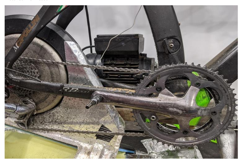
End of main test at 6000km – you will have less build up on chain rings than this, the standard test protocol had re-waxing more frequently than would be required in your real world riding, and that excess can be brushed off with a stiff bush in all of 30 secs if you do end up with more excess than you want. It is a very easy bush off clean, as opposed to concrete like waxes (Wend wax).
