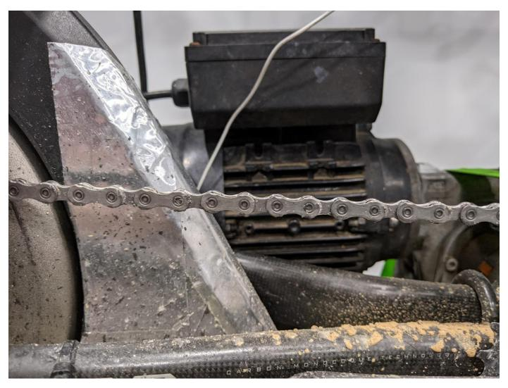
You can see the chain itself, again after 6000km of testing and a lot of contamination thrown at it, still looks brand new, with ZERO cleaning. And, at the end of all of that, it had only used up 1/3<sup>rd</sup> of its wear allowance.
