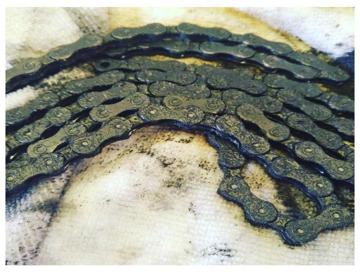
For fun lets compare that to the chain from the worst lubricant tested to date, Muc-Off Nano, which had used up 145% of its wear allowance after just 2000km. Can you spot the difference.....
