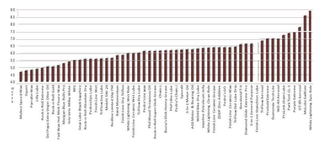
So, from the FF test information above, we have 49 lubricants out of 55 tested recording lower outright efficiency losses vs fastest factory grease at the time, and all 55 faster than the slowest factory grease at the time. And there are some truly
