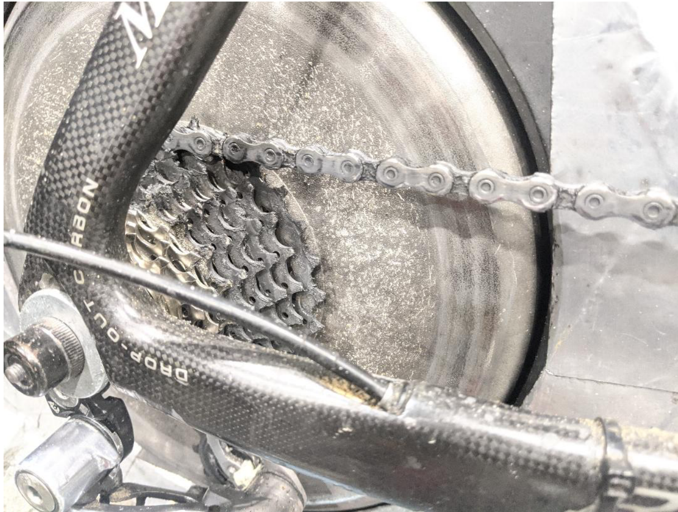
End of main test and end of wet contamination block 4 – 4000km.
