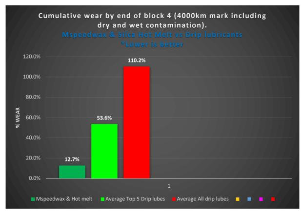
Again the above graph is at the 4000km mark in the main test, and includes a 1000km dry contamination block, a 1000km wet contamination block, and 2 x 1000km clean blocks with no contamination (set re lube / re wax points are done throughout test)
