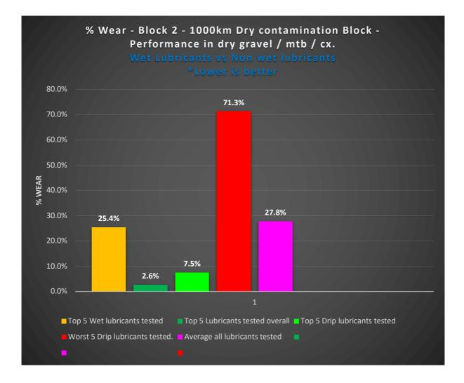
Alrighty, hopefully the above data really helps drive home the preceding bullet points. It is of course very handy that objective testing results lined up nicely with both the laws of physics as well as basic logic re what is happening if you head out with a wet lubricant into the world of dirt and dust.
