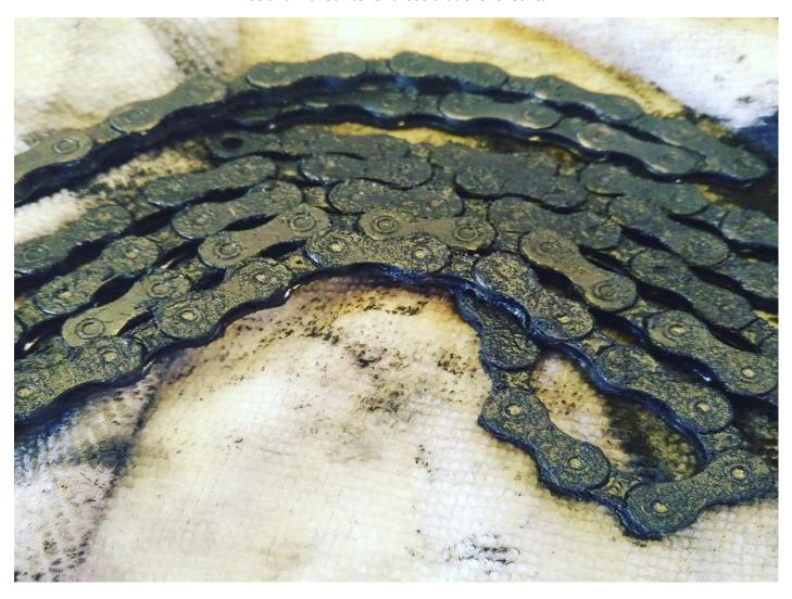
Ok finally - Below is my personal mtb drivetrain post the 213km XC marathon event using Silca Hot Melt. Overall this drivetrain is now 3400km old at time of picture, and I have never, ever cleaned the cassette except for jet wash post full mudders.
