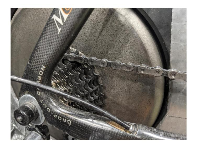
ON the plus side, things look better vs Muc-Off Nano chain after just 2000km!! This remains still, by far, the highest wear rate test, recording 145% of wear rate allowance by just the 2000km mark. Test stopped, and with chain looking like a coherent joining of black sludge – this lubricant proved not to be a fan favourite for those that ever tried it!
