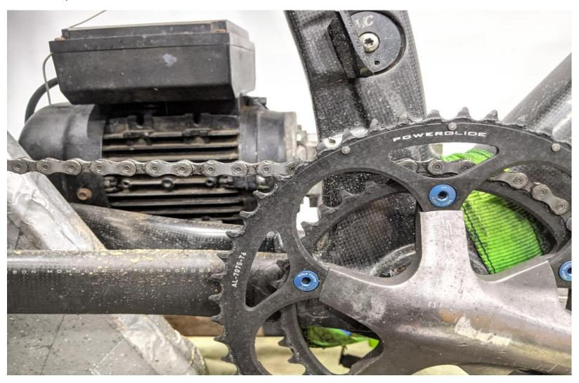
Revolubes post wet contamination block – 4000km into test
