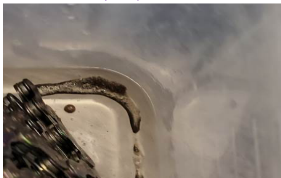
A lot of abrasive contamination no longer running in chain, or being brought into wax pot
