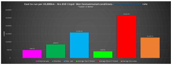
Immersive wax data does not include AB Graphenwax as that one product throws out the results for the other 5 immersive waxes tested by too much. With wet lubricants there is a much greater average spread
